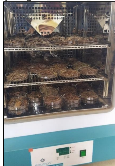
Sample fuel load prepared for estimation of oven dry weight
