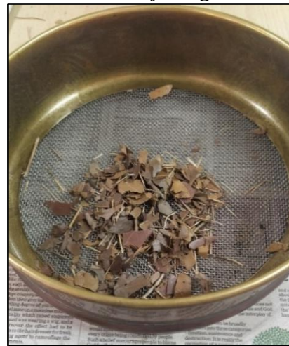
Crushing of fuel load for estimation of oven dry weight
