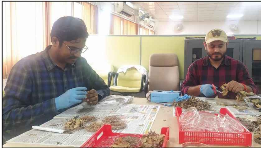
Surface Fuel Load being prepared for estimation of oven dry weight
