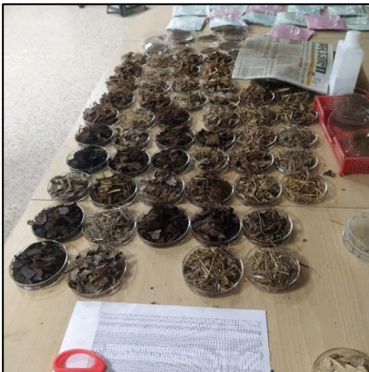
Sample fuel load prepared for estimation of oven dry weight
